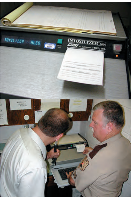
Sergeant Mike Kirby simulates a sobriety test with the Intoxilyzer 5000 machine. The computerized equipment uses a suspect's breath to analyze blood alcohol content.
